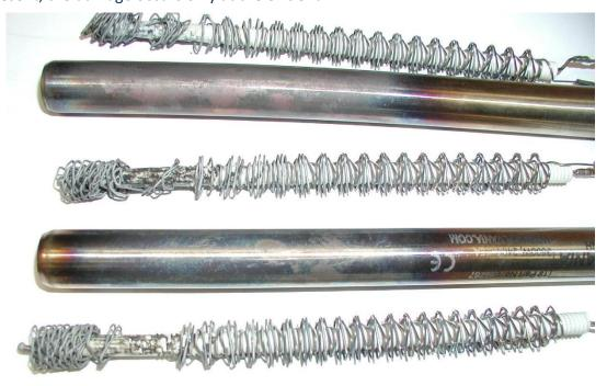
B) Failure due to applied voltage with zero airflow. Note damage occurs along entire length.
